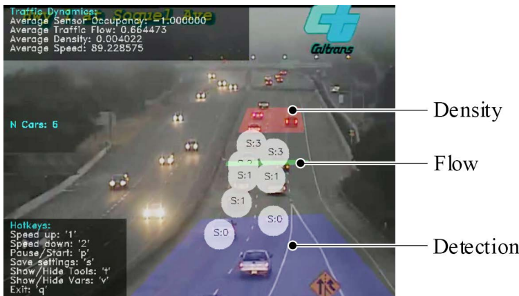
Figure 1. Example of a Traffic Dynamics Meter (TDM). This TDM detects vehicles (blue zone), estimates traffic flow (green zone), and determines traffic density (red zone), as traffic speed is computed alongside these zones. This road feed corresponds to Soquel Ave in Santa Cruz, California. (California Department of Transportation (Caltrans)). Note: Caltrans Streaming Video Locations. Caltrans. Retrieved (2018).
